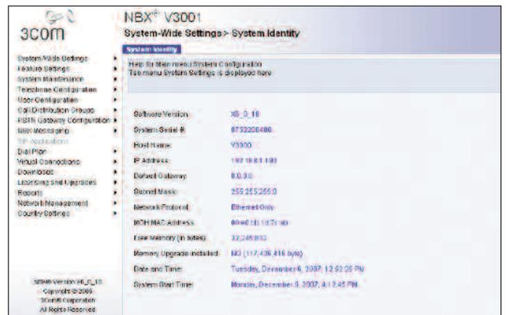
The NBX NetSet management interface provides point-and-click setup for the most basic or the most complex telephony features.
